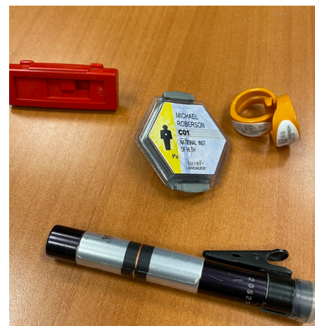
Dosimeters come in all shapes and sizes. Clockwise from left: film badge holder that can fit on a wristband, badge to measure whole-body radiation exposure, two ring dosimeters, and pocket dosimeter.
